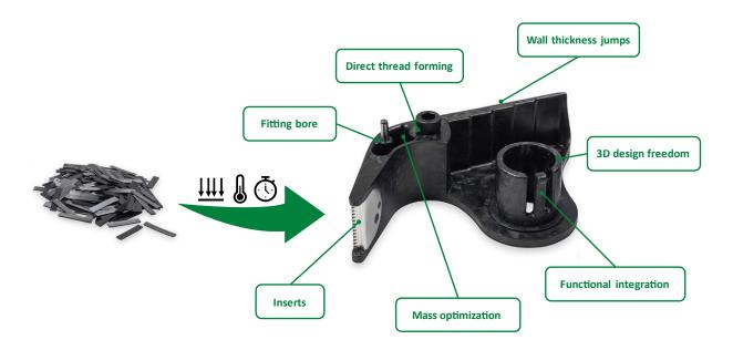
Automated production ensures high reproducibility in series production and, depending on the size of the component, achieves a manufacturing volume of up to 100,000 components per year. In contrast to thermoset matrix systems, a complete recycling of the fiber chips by means of highvoltage fragmentation is possible. The chips can then be returned to the aCC process.
